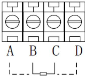
Note: two wire heating resistors are connected to BC terminal, while AB is connected to CD.
