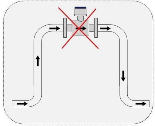
Install at the lowest point when used in open drain pipe
