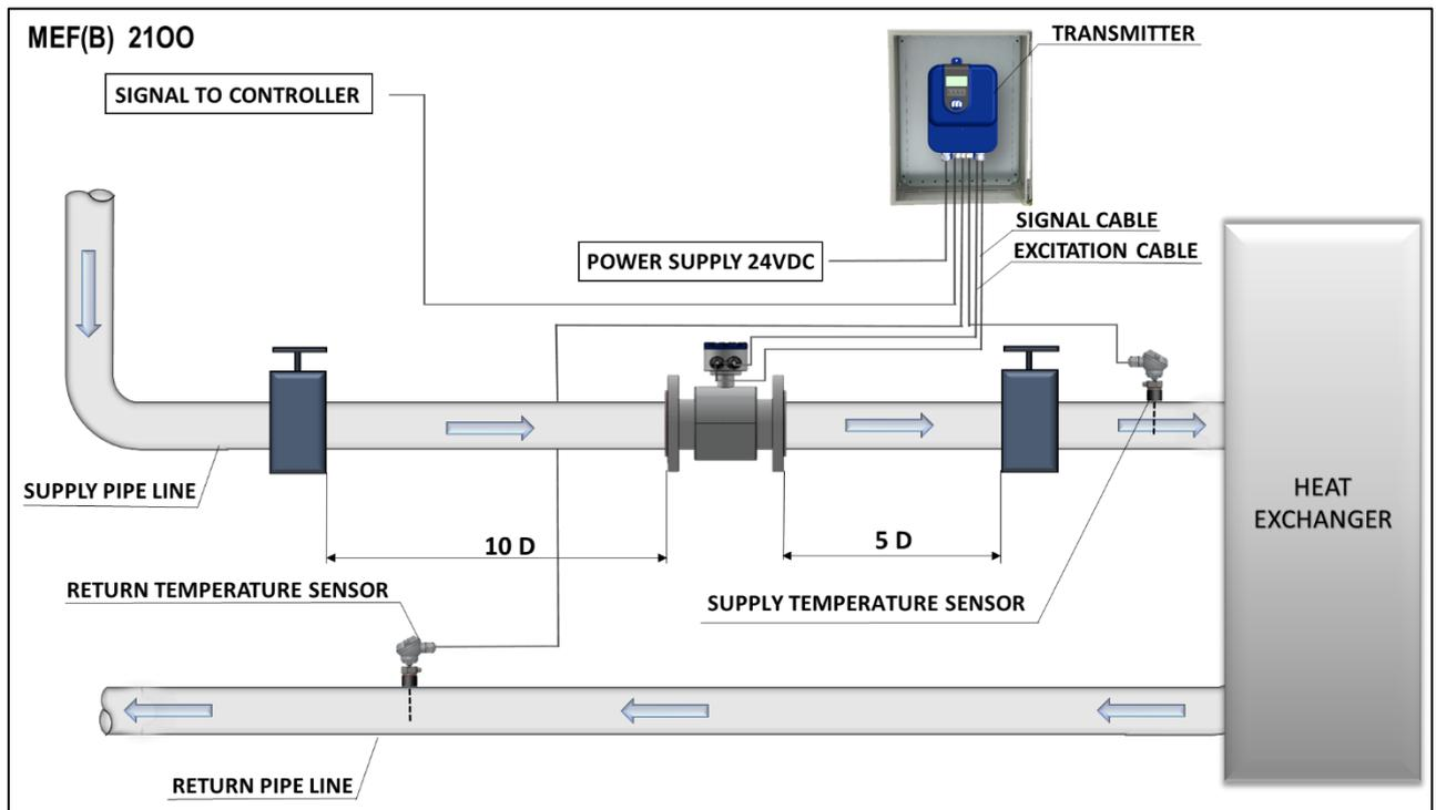
To ensure electromagnetic BTU meters work correctly, install the flow sensor head at the top of a horizontal pipe at the 12 o'clock position. The pipeline must be pressurized and filled entirely with clean water, without any air or particles. Air and particles act as insulators, disrupting the meters' electromagnetic induction and impairing their function. For vertical pipes, install the meter so water flows from bottom to top for optimal performance.
