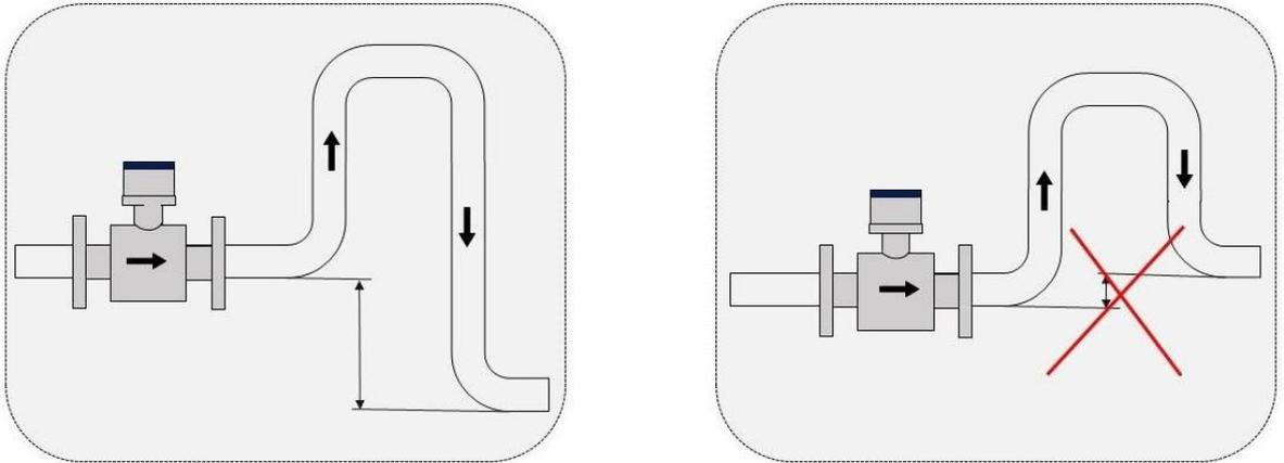
The downstream of BTU meter when the drop is more than 5 m
