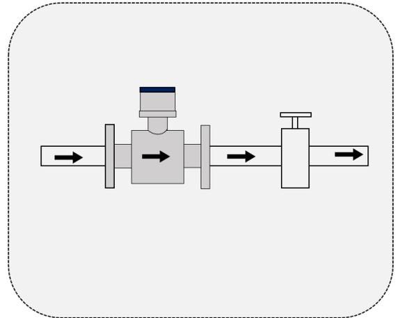
Don't install it at the exit of the valve, install it at the entrance of the valve
