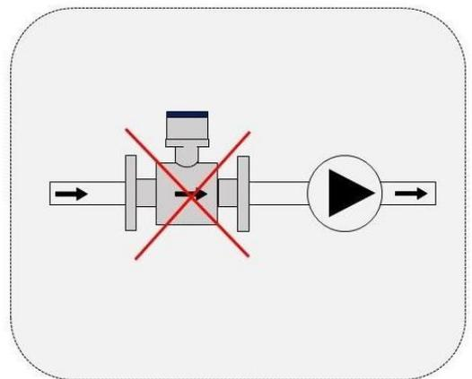
Don't install it at the entrance of the pump, install it at the exit of the pump
