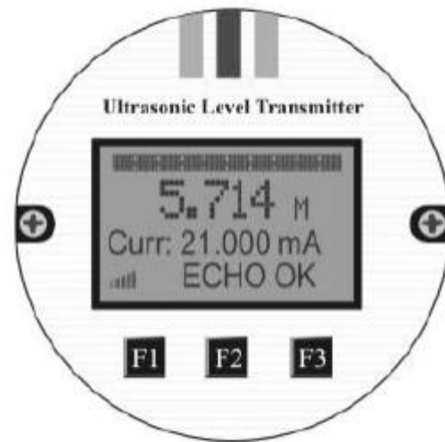
LCD display screen after opening the cov
