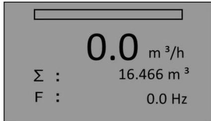
Press "Z" button, and then press "S" button to find menu "Unit Qv" (This is to set volume flow unit)
