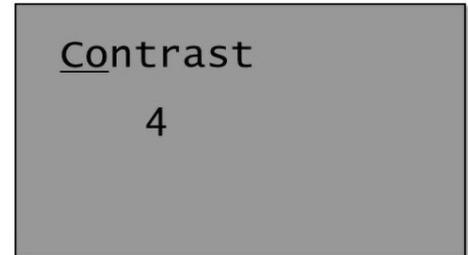
Press "M" button for 2 seconds to enter into this menu press "S" button to chose the option
